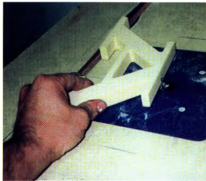
17. Edges of the secondary copy were routed using a ¼-in. round-over bit
