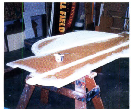
15. Priming the raised border
