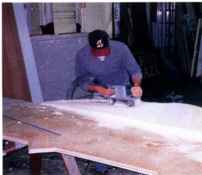
7. Rough shaping the train with the belt sander
