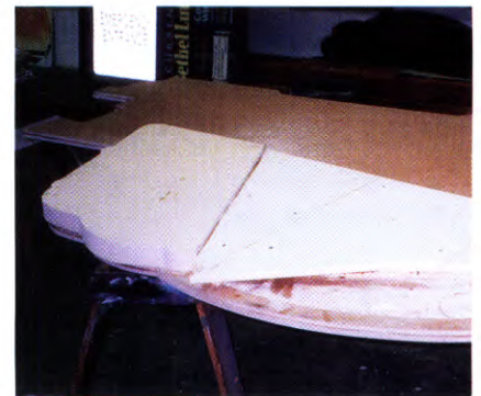
6. Gluing high-density urethane panels up for train graphic
