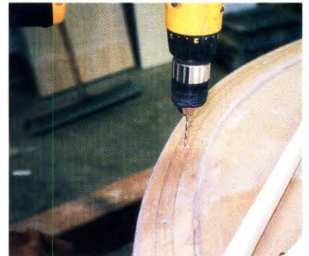
12. Predrilling for the top border section
