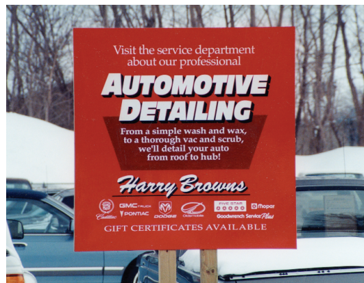
Vinyl lettering on a 3-by-4-ft. panel of 1/2-in. overlaid plywood
