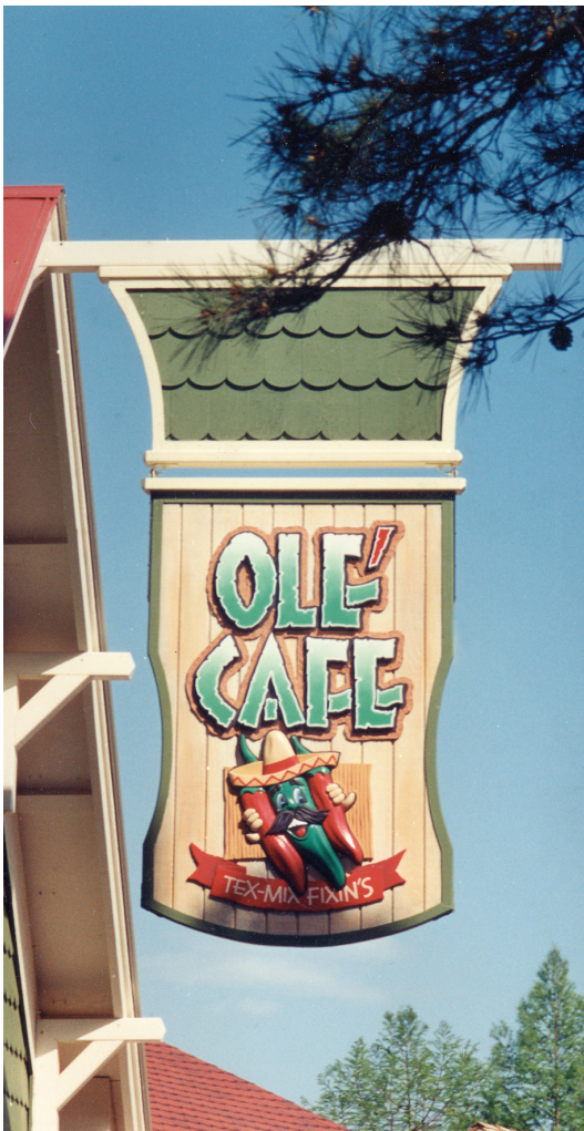
Enamel on 3-by-6-ft. cedar siding and panel, finished with acrylic latex paint; the carved peppers, cutout letters and banner are high-density urethane board
