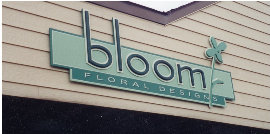
High-density urethane board on 4-by-10-ft. overlaid plywood panel, finished with acrylic latex paint
