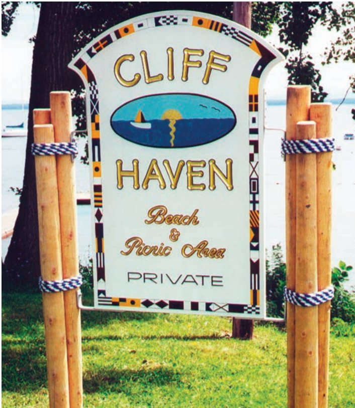
4-by-6-ft. panel of 3/4-in. high density urethane board laminated to 1/2-in. overlaid plywood. "The border is the actual nautical alphabet, A to Z," says Bob, and there are two hidden messages in the border." Lettering is 23k gold leaf; paint is 1-Shot [219-949-1684, www.1shot.com] enamel and acrylic latex. Posts are cedar, wrapped with nylon rope.
