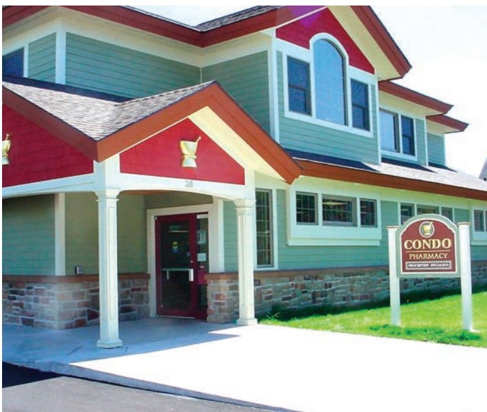
Double-faced 48-by-52-in. sign on 6-by-6-in. posts. The faces are hand carved 3/4-in HDU laminated with epoxy to 1/2-in. overlaid plywood. The background behind graphic is coarse white smalts “drowned” in dark green acrylic latex paint and Smith’s cream. The carved lettering is gilded.
