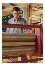
We laminated the panels with 3M neoprene-base contact cement, giving them a few really tight squeezes with a professionally made pinch-roller. If you don't have a good pinch-roller, stick with epoxy. It has better gap-filling properties.
