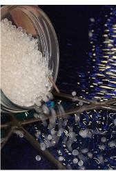
A tablespoon of silica desiccant beads was used on each side of the leaded glass. The sign is up high so the little pile of beads cannot be seen from street level.
