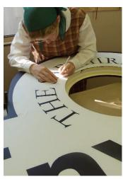
After applying three coats of acrylic latex paint, the panel was masked and weeded. We usually finish first and carve through a mask.
