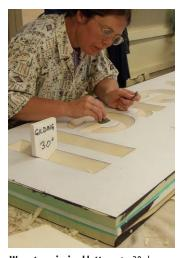
We cut our incised letters at a 30-degree angle when they will be gilded, and at a 35-degree angle if they will be painted. The deeper cut yields more striking shadows on painted letters. Here you can see the template used for checking the angle.
