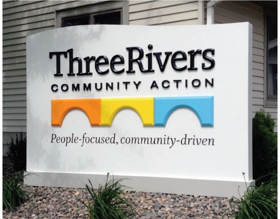
HDU letters and graphics, cut on the ShopBot CNC router then mounted on an aluminum composite panel with an aluminum tube frame, finished with exterior acrylic paints.
