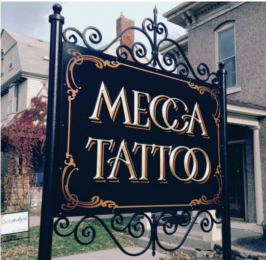
Letters were cut on the ShopBot CNC router then mounted on an aluminum composite panel with an aluminum tube frame. Letters are finished with 23K gold leaf.
